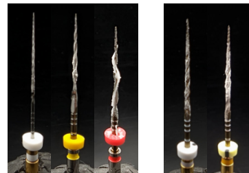
Fig 2: Comparative image of the files after debris removal to illustrate the differences in cutting performance
